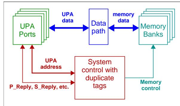
To allow scaling beyond traditional snoopy buses, the UPA defines a point-to-point packet-switched protocol between the distributed system control function. For example, the sequence for a load-miss to memory is:
