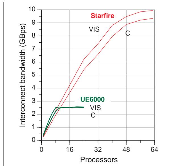
The VIS assembler code is more latency tolerant than the C code, which was compiled with a version of the compiler that did not generate software prefetches. The VIS bandwidths rise somewhat faster to the peak bandwidths. We observed bandwidths up to 97% of peak on the Starfire, and up to 99% of peak on the UE6000.
