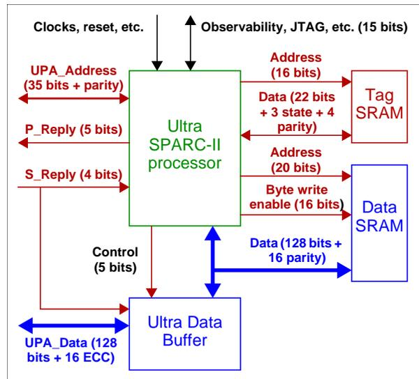
The processor can execute four operations per clock, including one floating-point multiply and one floating-point add. It supports software-initiated prefetches. There may be up to three outstanding memory transac-
