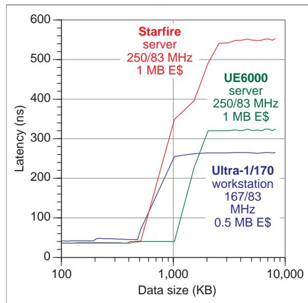
Memory latency is shortest for the workstation, because that system is small enough to fit on one board, and there
