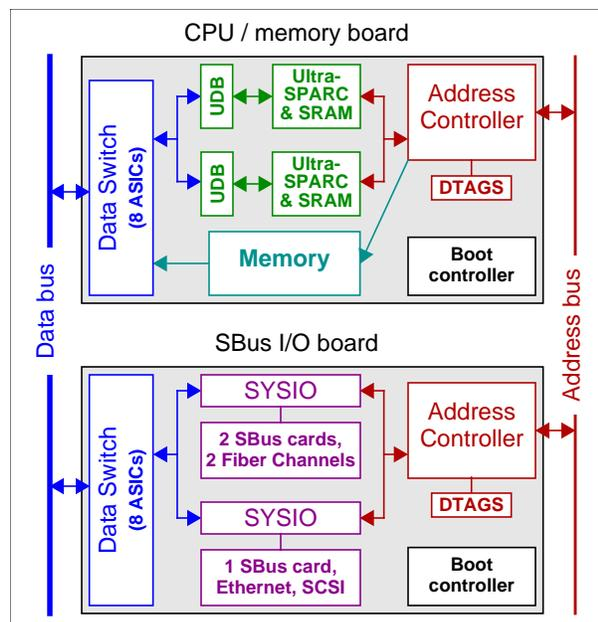
The UE6000 is implemented with eight board slots on either side of its centerplane. Smaller cabinets (UE4000 and UE3000) hold eight and four boards respectively. The boards are 11.5" x 10" in size, and have a 2" spacing on the centerplane.
