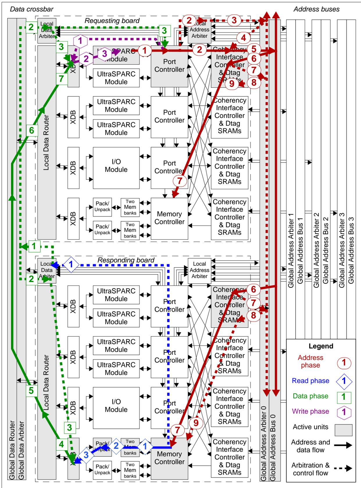
6. The **Global Data Router** sends the data to the destination Local Data Router.
