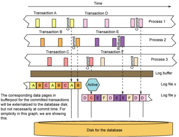
This figure shows several transactions running over a period of time. Some transactions run concurrently; they start filling up the log buffer first, and are subsequently written to the log files on disk.
