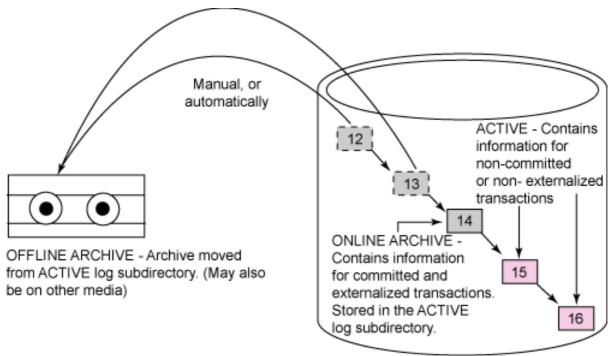
The type of logging for a database is determined by the database parameter LOGARCHMETH1. When LOGARCHMETH1 is OFF (default), archival logging is disabled, and circular logging is used.
