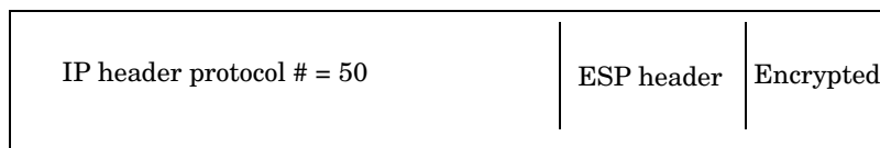
Figure 9-6 Packet with IPSec-Encrypted TCP Data
