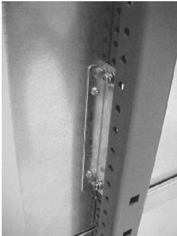
**Step 5.** Secure the ICE to the mounting brackets using the two captive screws.
