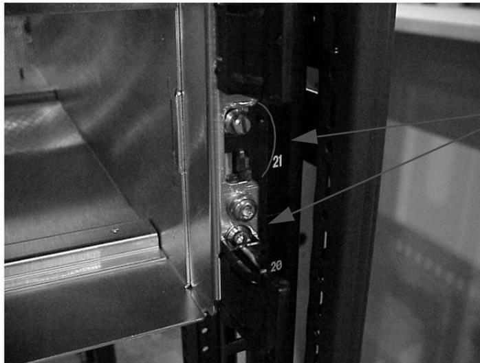
Observe the clearance features for the 10KG2 rack universal rail pins.
