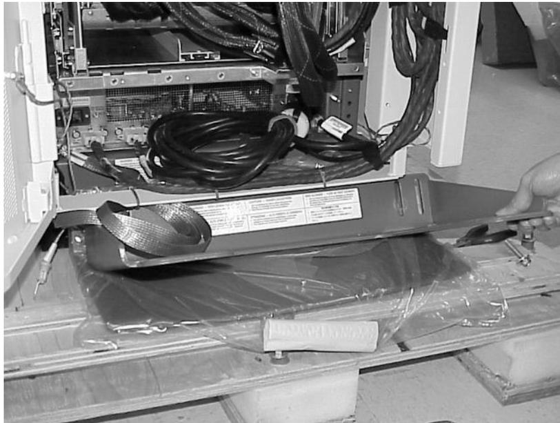
**Step 8.** Remove the power cord from the cabinet back rail by cutting the green tie-wraps on the rail and removing the green VELCRO ties holding the cord.
