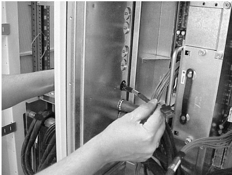
**Step 4.** Determine which shield protector to remove and pull the perforated section. Discard the plastic.
