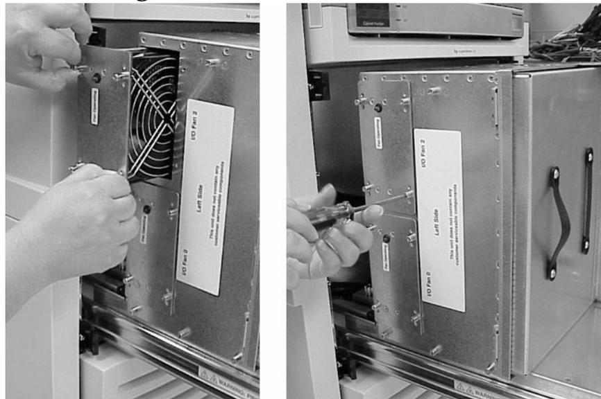
**Step 3.** Disengage the ICE slide rail locking tabs and slide the ICE into the rack.
