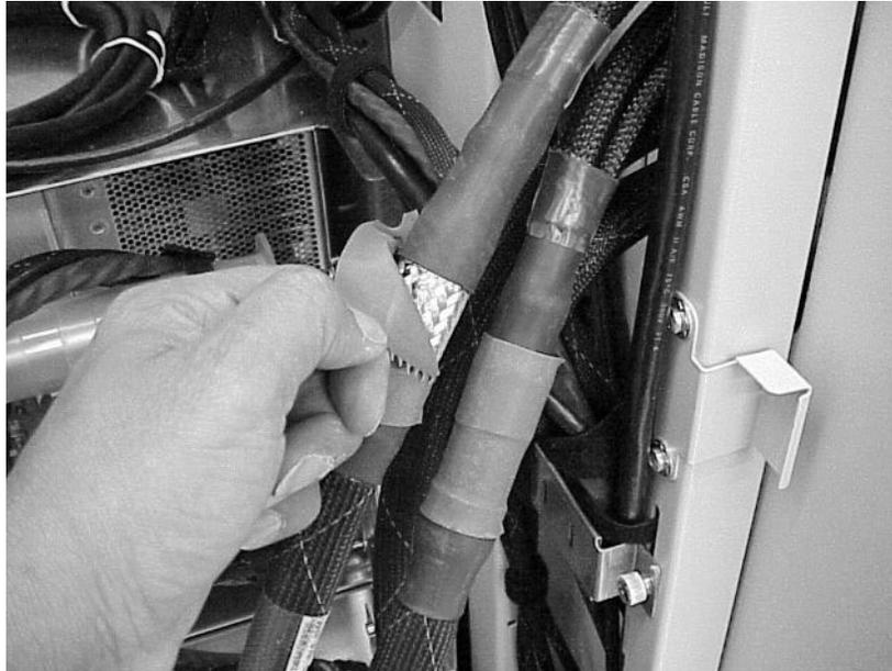
**Step 7.** Separate the halves of an R-PEC. You will have to loosen the screws in the blanks to facilitate their removal.
