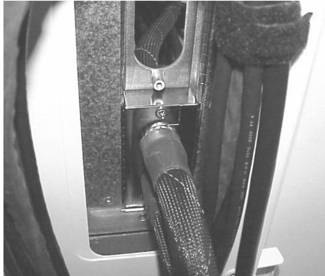
**Step 10.** Connect the REO cable to the appropriate Cell board connector in the Superdome server.
