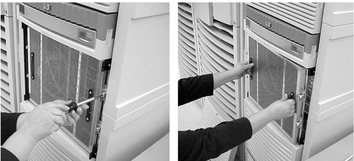
Removing and Replacing the ICE I/O chassis
