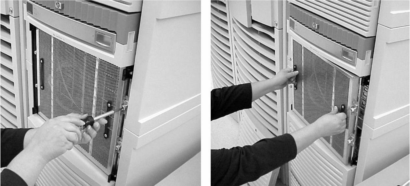
**Step 4.** Disengage the lock pins and slide out the ICE on its tray.
