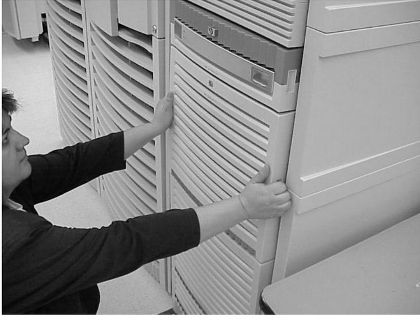
**Step 4.** Remove the EMI panel from the ICE by loosening the four captive retaining screws and pulling the panel off.
