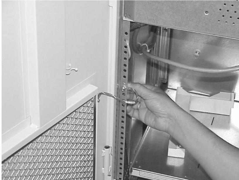
3. Remove the rear door. Turn the door inward and lift it off its three hinges.
