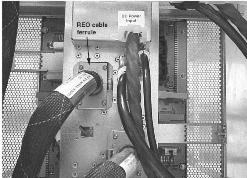
**Step 5.** Push the REO cable connectors into their respective connectors on the XMIOB.
