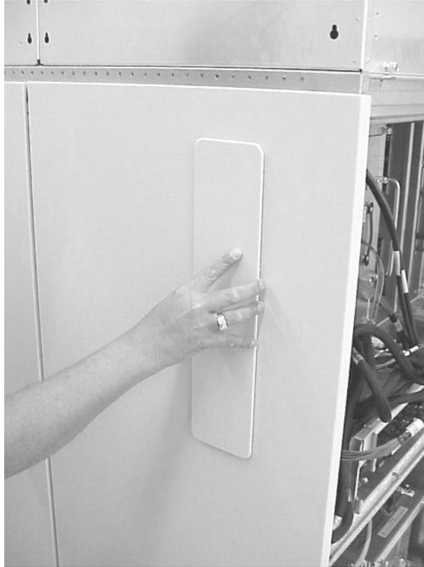
**Step 2.** Remove the IOX exit panel blank on the side that is to be next to the Superdome server.
