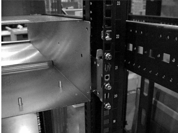
Installing the ICE Enclosure into the Rack
