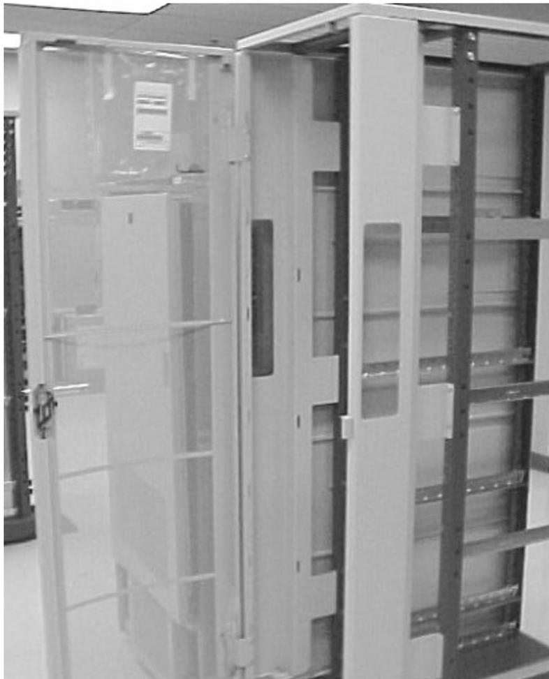
The top cap is 16-gauge, cold-rolled steel (CRS). The top cap and forehead are attached at the factory. The top of the cabinet incorporates a ventilation path through the roof of the cabinet and a convection current heat exit for the heat generated by the installed equipment.
