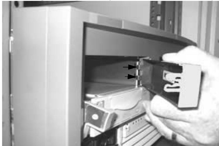
**Figure A-13 Tape Array Front Bezel and Vacant Drive Bay Bezels Installed**
