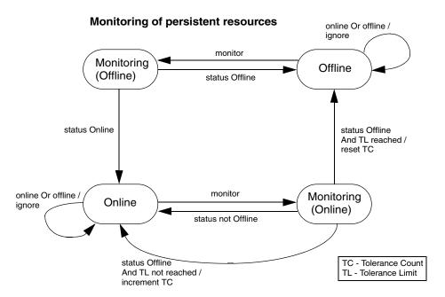
For a persistent resource in the Online state, if <code>monitor</code> returns a status of offline and the <code>ToleranceLimit</code> is not reached, the resource stays in an Online state. If <code>monitor</code> returns offline and the <code>ToleranceLimit</code> is reached, the resource is placed in an Offline state and noted as <code>FAULTED</code>. If <code>monitor</code> returns "not offline," the resource stays in an Online state.
