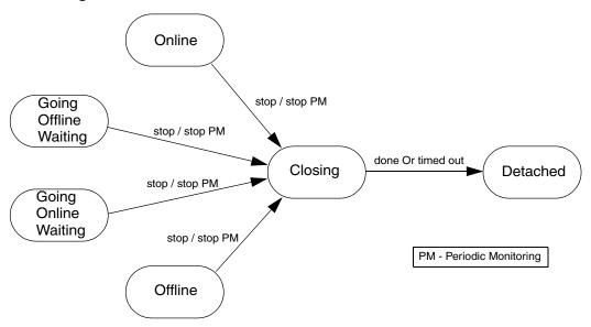
When the resource is disabled (Enabled=0), the agent stops Periodic Monitoring and the the close entry point is invoked. When the close entry point succeeds or times out, the resource is placed in the Detached state.
