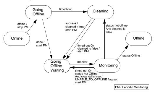
Upon receiving a request from the VCS engine to offline a resource, the agent places the resource in a Going Offline state and invokes the <code>offline</code> entry point.
