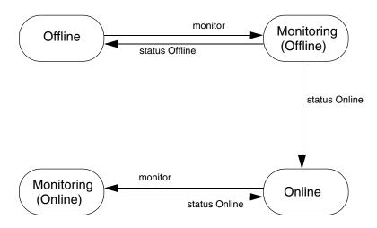
When resources are in a steady state of Online or Offline, they are monitored at regular intervals. The intervals are specified by the MonitorInterval parameter for a resource in the Online state and the OfflineMonitorInterval parameter for a resource in the Offline state. An Online resource that is unexpectedly detected as Offline is considered to be faulted. Refer to diagrams describing faulted resources.
