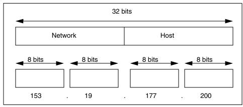
Figure 3-1 IP address format
