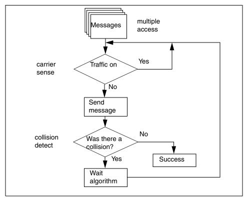
Figure 2-2 CSMA/CD algorithm
