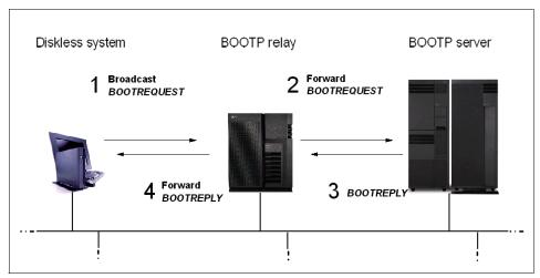
Figure 6-1 The BOOTP client/server message flow
