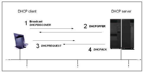
*Figure 6-2* The DHCP client/server simple request message flow
