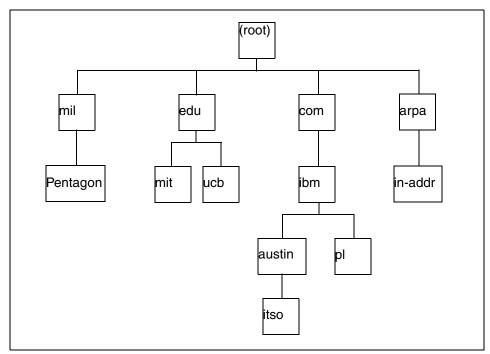
Figure 8-1 DNS structure
