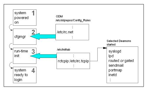
Figure 5-1 TCP/IP network startup procedure
