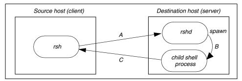
Figure 4-9 Execution process flow of rsh
