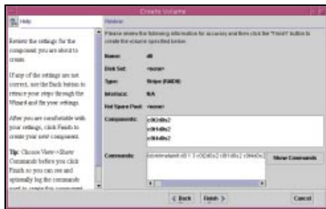
Figure 13. The Review step shows you the particular type of volume and RAID level Solaris will create.
