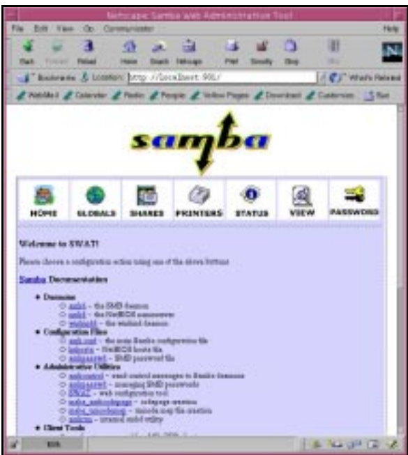
Figure 21. On the SWAT page you can get to different parts of the SAMBA configuration routine by clicking on the buttons across the top of the screen, and view configuration information by clicking on the links in the main body of the page.
