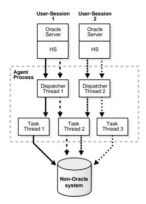
These three thread types roughly correspond to the Oracle multithreaded server's PMON, dispatcher and shared server processes respectively.
