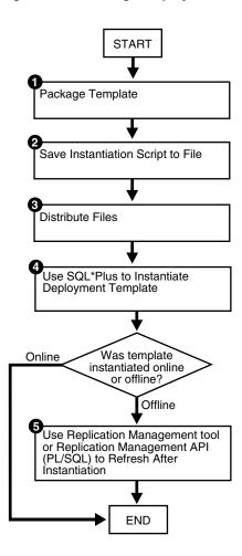
Figure 4–2 Packaging and Instantiating a Deployment Template
