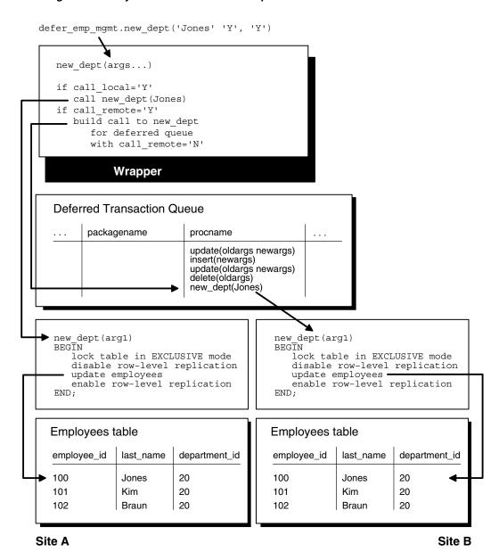
Figure 7-4 Asynchronous Procedural Replication
