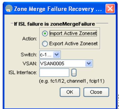
Figure 26-29 Zone Merge Fail Recovery
