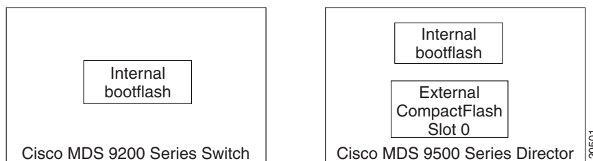
Figure 14-1 Flash Devices in the Cisco MDS 9000 Supervisor Module
