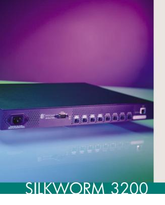
The Brocade SilkWorm 3200 Entry Fabric Switch simplifies Storage Area Network (SAN) deployment, enabling cost-effective migration from Direct-Attached Storage (DAS) environments.
