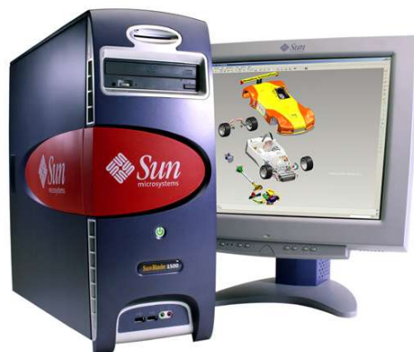
Sun Blade 1500 1 GHz USIIIi CPU
