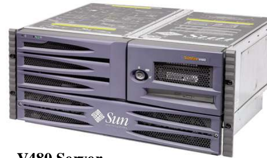
V480 Server 4 USIII CPU's - 1.2 GHz 32 GB memory 2 internal 73 GB Disks
