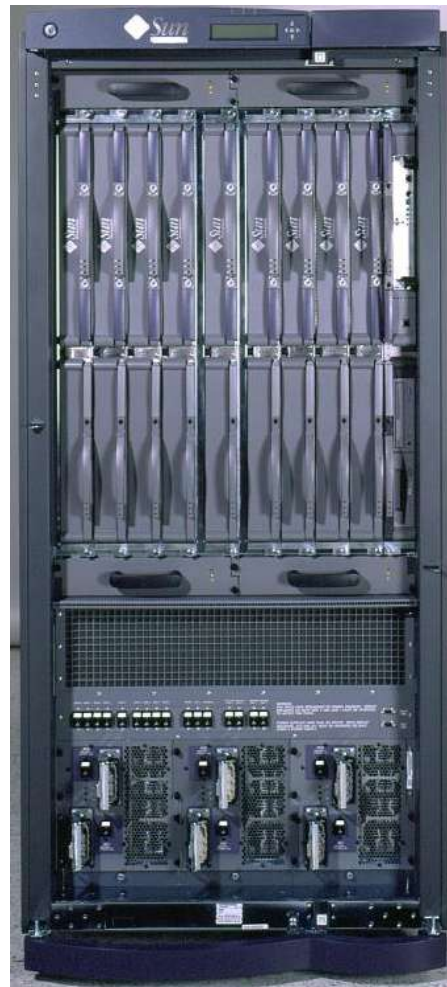
Sun Fire E25K Server 72 USIV CPU's 576 GB memory 18 domains
