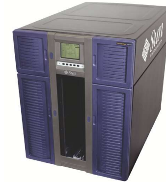
L100 Tape Library Drives: 6 SDLT320 or 6 LTO Cartridges: 100 SDLT320 or 84 LTO
