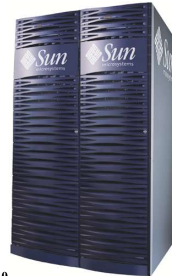
6320 11 6120 Arrays Dual 16 port 2 GB Switches 1 Service Processor 45 TB 22 GB Cache
