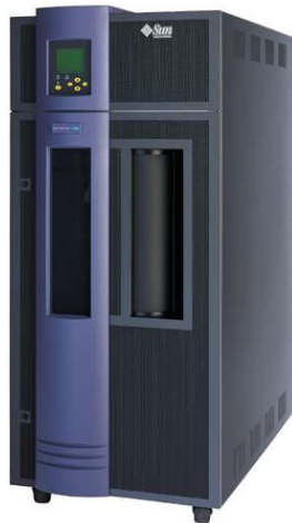
L180 Tape Library Drives: 10 SDLT320, 10 LTO2 or 6 9840 174 Cartridges
