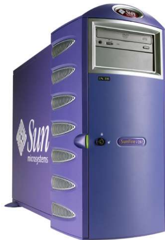
V250 Server 2 USIIIi CPU's - 1.28 GHz 8 GB memory 8 internal 73 GB Disks
