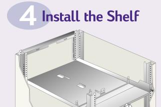
From the back, slide the shelf into the rack until the front lip is over the bezel. Slide the rear lip over the clipnuts on the back rails. Tighten the screws in the bottom clipnuts. Install and tighten two 10-32 screws in the top clipnuts.
