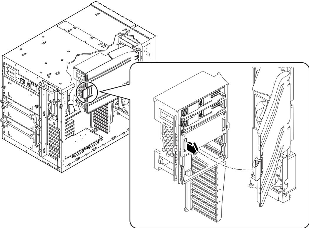
**2. Unhook the air guide tabs from the CPU fan tray assembly.**
