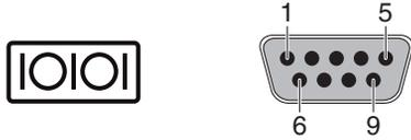
**FIGURE 4-4** Serial Port Pin Numbering
