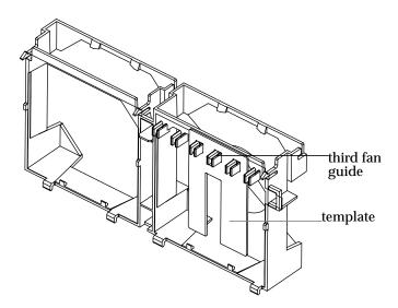
Note - Place the template so that the middle square of the template fits into the third fan guide from the right.
