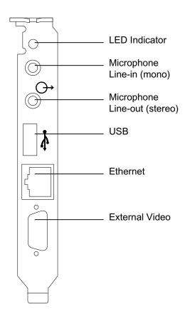
FIGURE 10-1 SunPCi III Main Card Backplate Connectors
