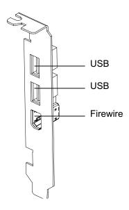
FIGURE 10-2 SunPCi III USB/Firewire Backplate Connectors
