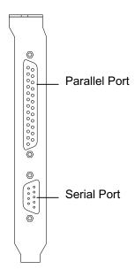
FIGURE 10-3 SunPCi III Serial/Parallel Port Backplate Connectors
