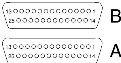
**FIGURE 11-3** DB-25 Serial Connectors**TABLE 11-2** Serial Connector Pinout, RS423/RS232
