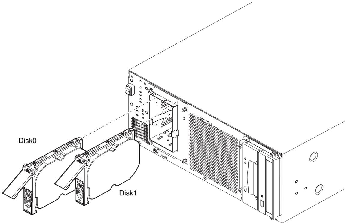
**FIGURE 8-1** FC-AL Disk Drive and Drive Bay Assembly
