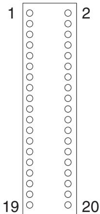
**FIGURE D-3** Internal FC-AL Connector, J2901
