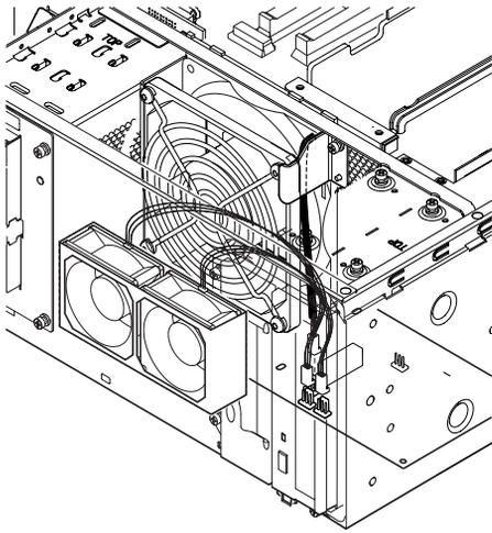
**FIGURE 7-4** Fan Connectors
