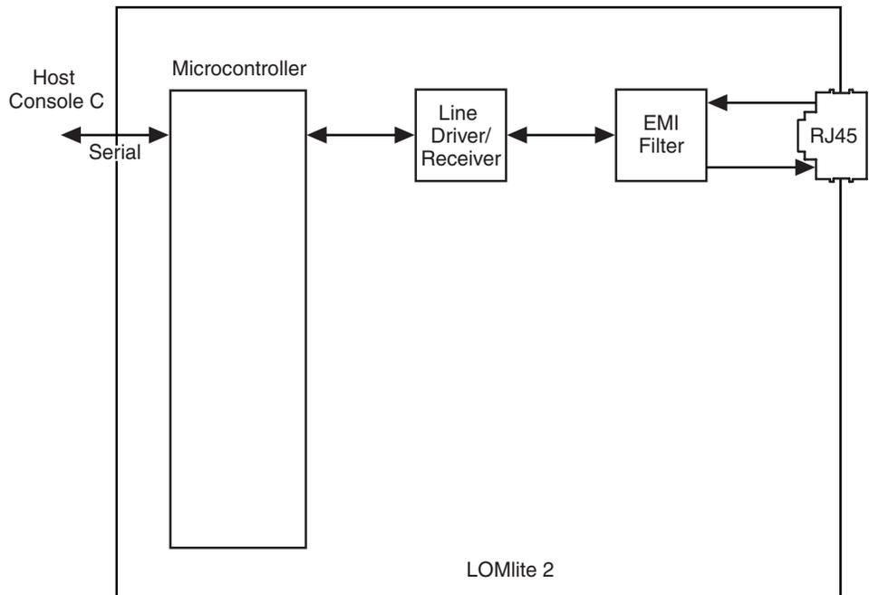
**FIGURE 10-15** LOMlite2 Serial Port Functionality
