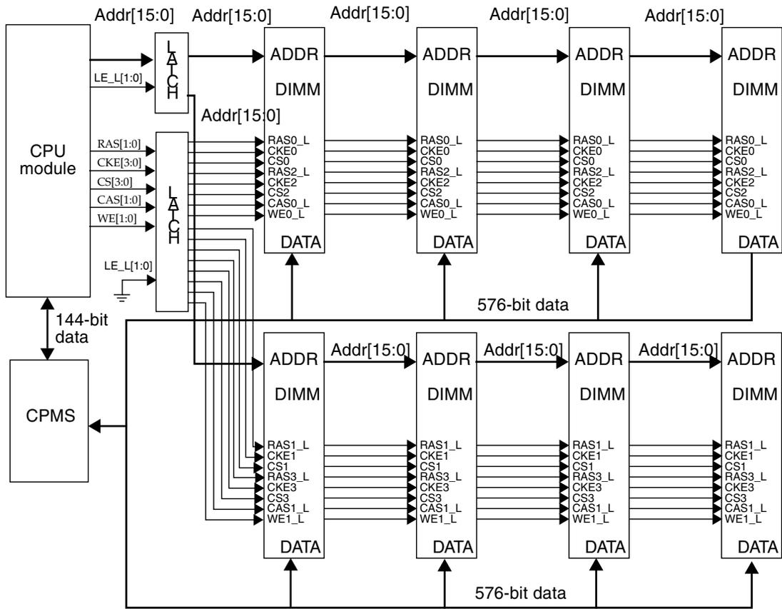
FIGURE 10-5 Main Memory Functional Block Diagram
