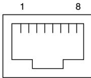
**FIGURE 11-10** RJ45 Lights Out Management Serial Connector
