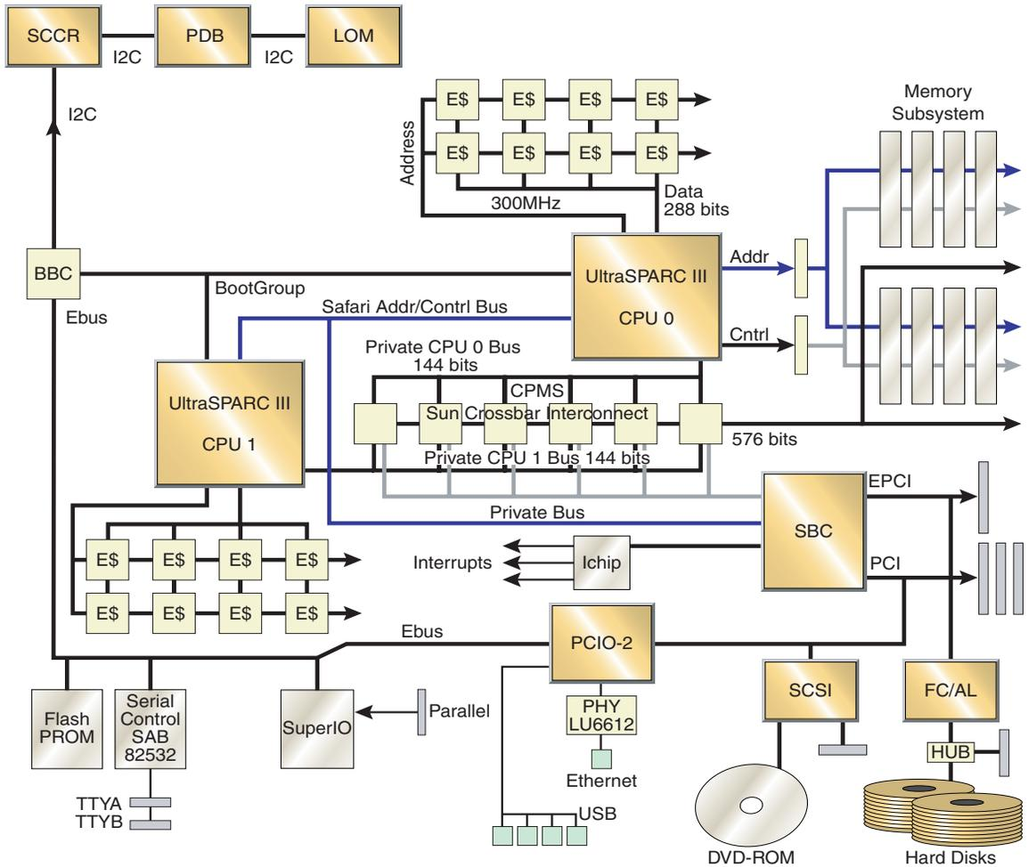
FIGURE 10-1 Netra 20 Logical System Diagram
