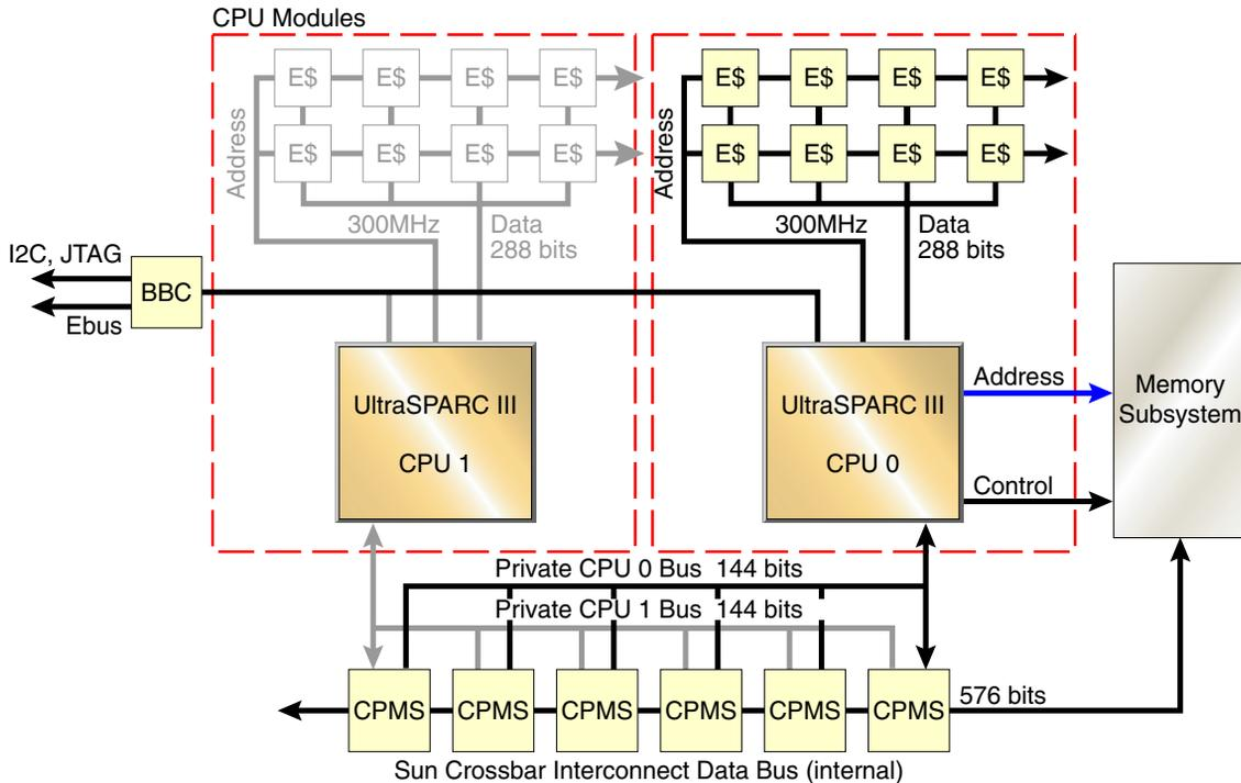
FIGURE 10-2 UltraSPARC-III Processor Functional Block Diagram
