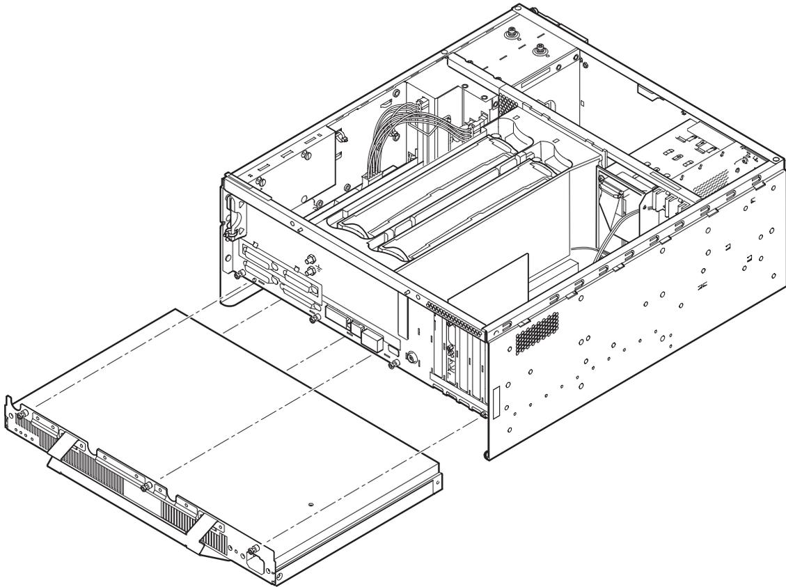
**FIGURE 6-1** Power Supply Unit
