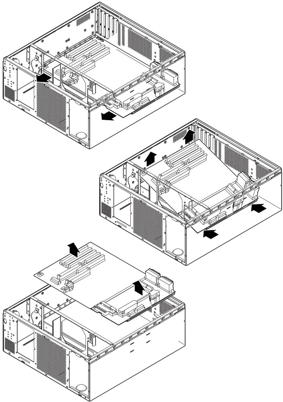
**FIGURE 8-11** Removing the Motherboard from the Chassis
