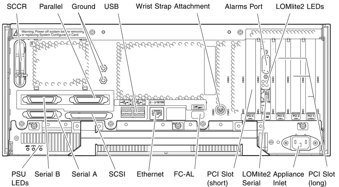
**FIGURE 11-1** Back Panel Connectors (AC Version Shown)
