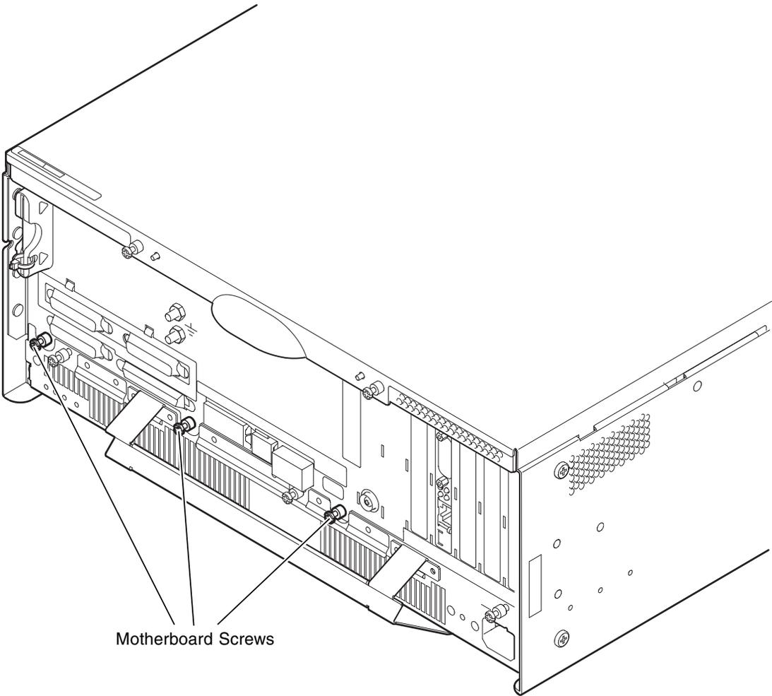
FIGURE 8-10 Motherboard Fixing Screws
