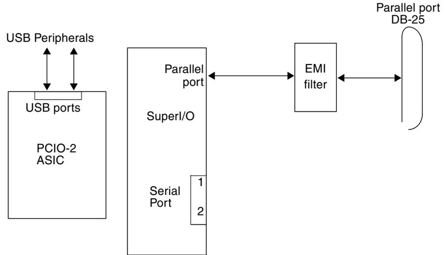
FIGURE 10-13 USB and Parallel Port Functional Block Diagram
