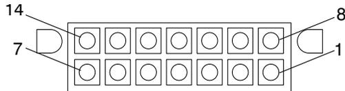
**FIGURE D-4** Power Supply Connector J3603**TABLE D-5** Power Supply Connector J3603 Pin Description
