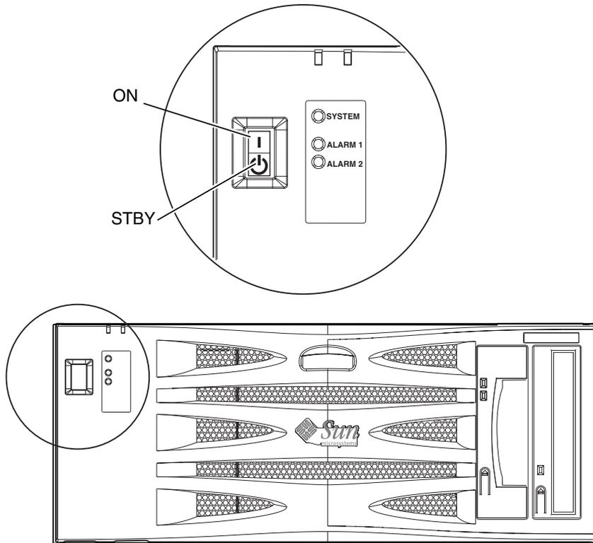
FIGURE 5-1 System Power On/STBY (Front Panel)
