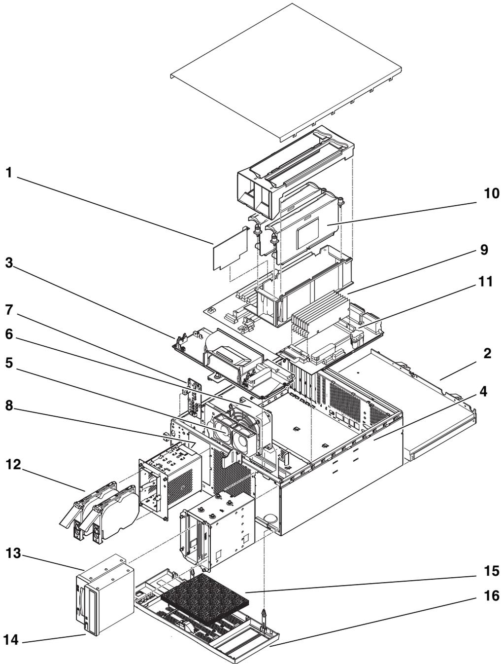
**FIGURE A-1** Exploded View of the Netra 20 System Unit
