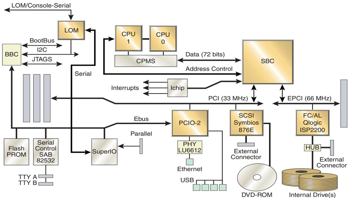
**FIGURE 10-3** I/O Logical Diagram
