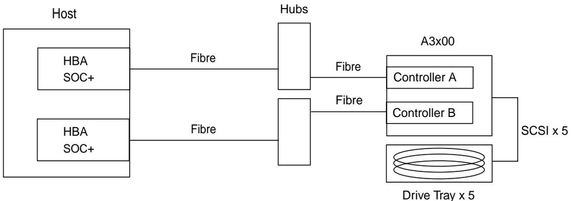
**FIGURE 2** Host Attachment Through Hubs—Single Array, Single Host
