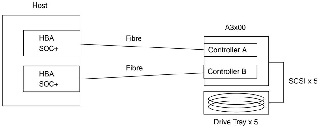
**FIGURE 1** Direct Host Attachment—Single Array, Single Host
