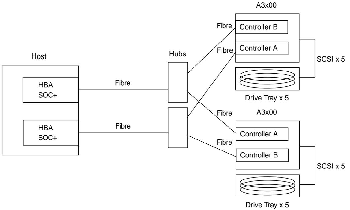
**FIGURE 3** Host Attachment Through Hubs—Multiple Arrays, Single Host
