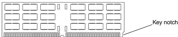
**FIGURE 2-5** DIMM—Front View
