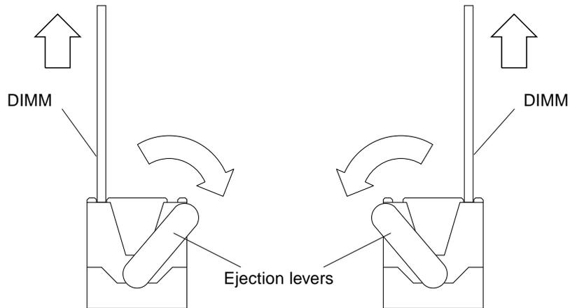
**FIGURE 2-7** DIMM Ejection Levers
