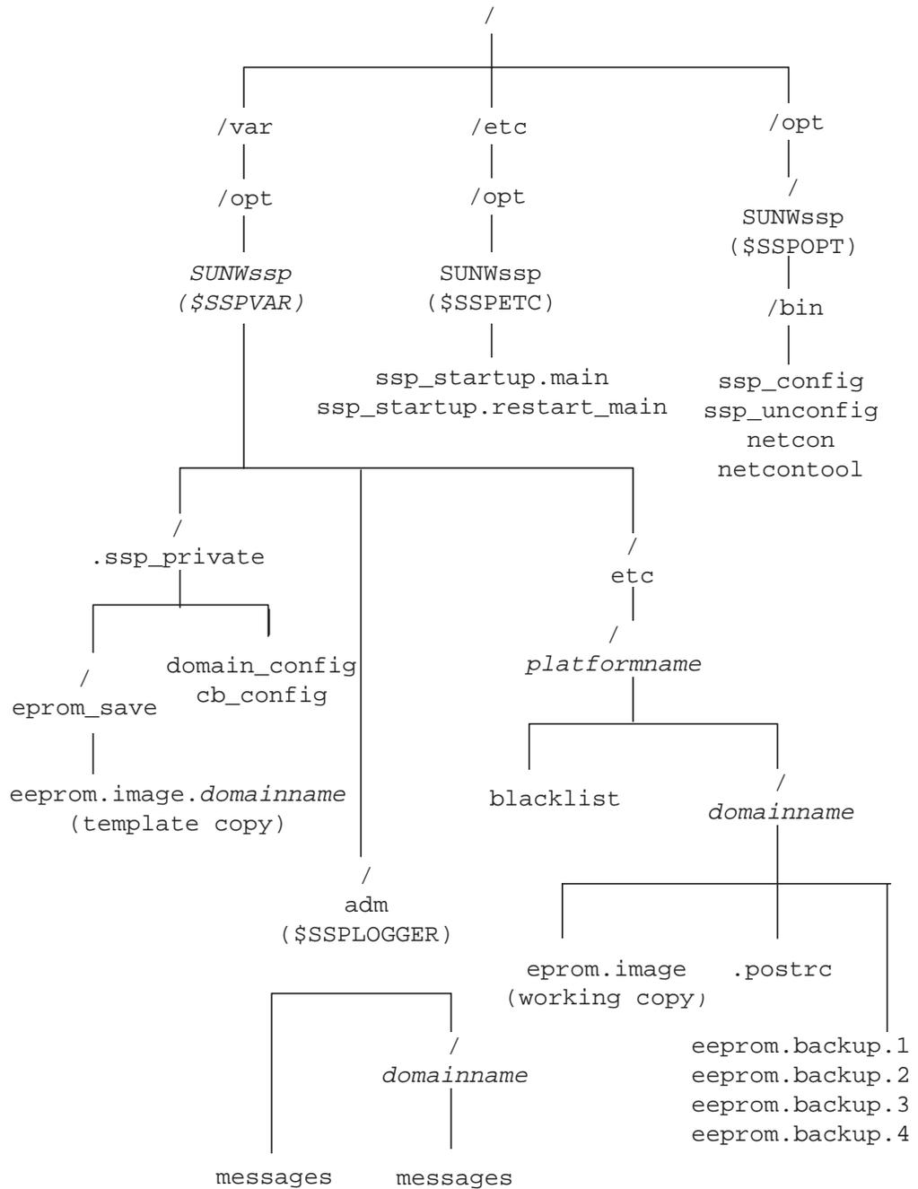
**Figure 3-6** SSP File System Structure
