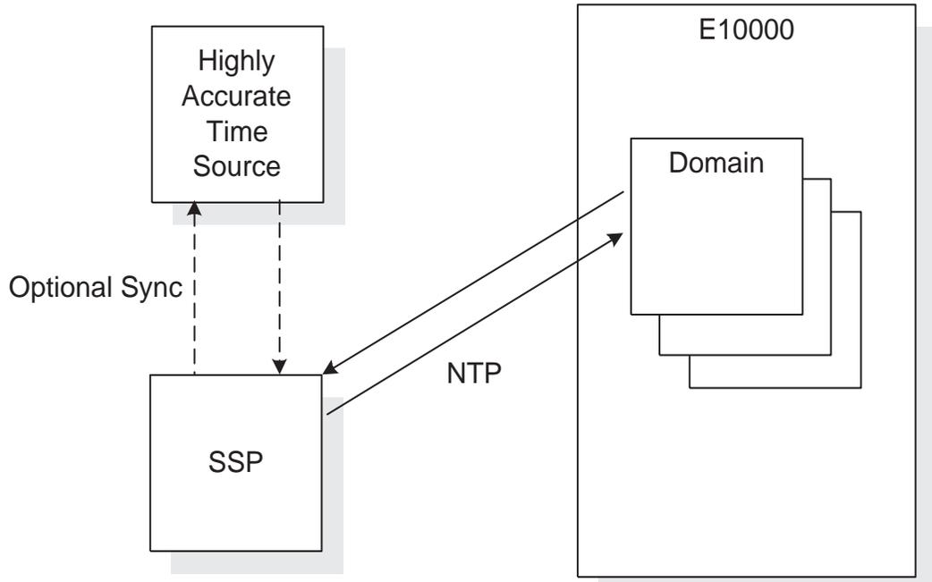
**Figure 3-13** Synchronizing Between SSP and the Domains
