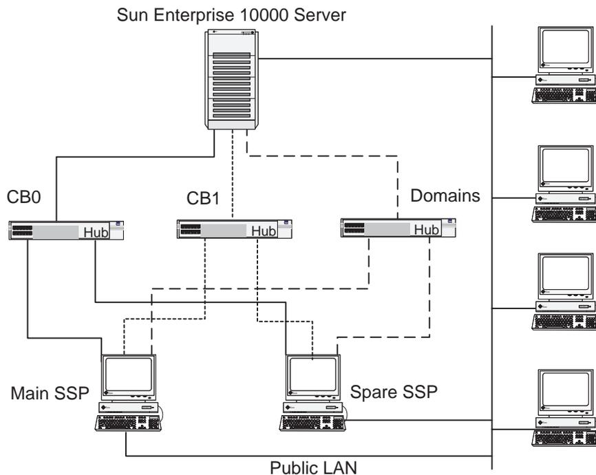
**Figure 3-1** SSP-to-Sun Enterprise 10000 Server Connectivity
