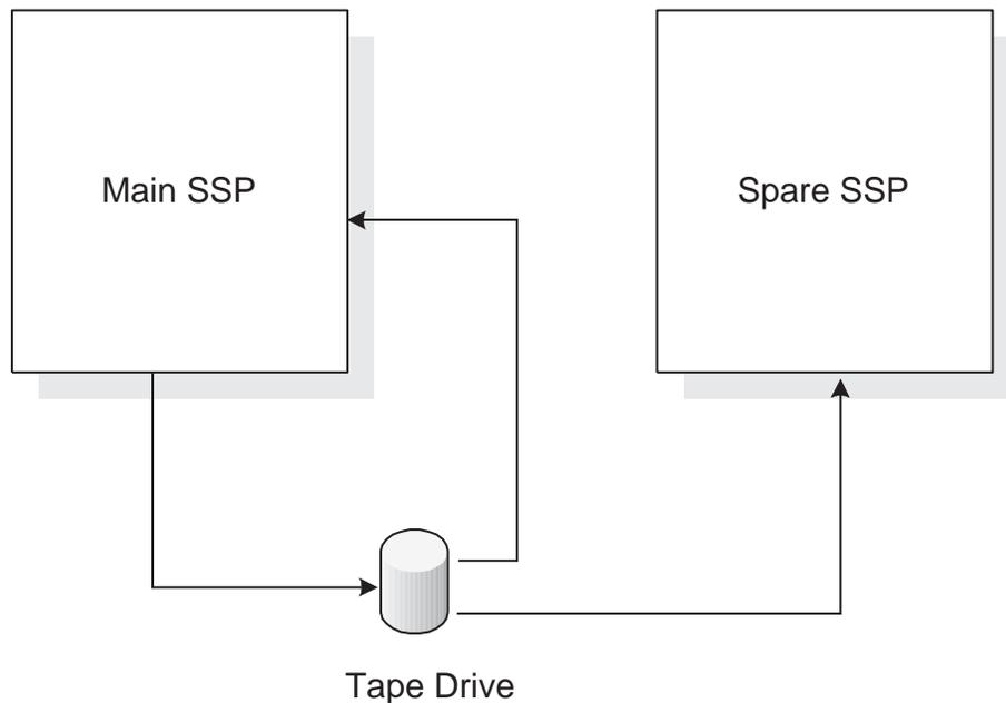
**Figure 3-12** Saving the SSP Environment
