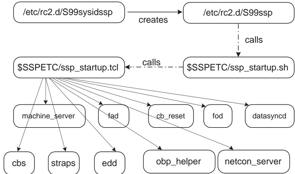
**Figure 3-7** The SSP Boot Process
