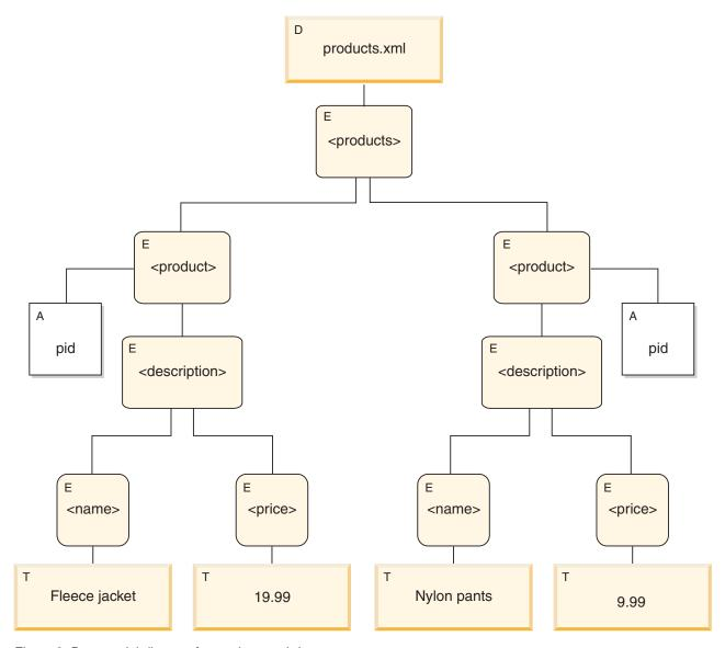
Figure 3. Data model diagram for products.xml document
