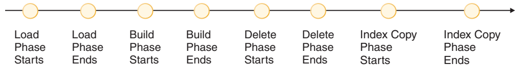
Figure 1. The Four Phases of the Load Process: Load, Build, Delete, and Index Copy. While the load operation is taking place, the target table is in the load in progress state. If the table has constraints, the table will also be in the set integrity pending state. If the ALLOW READ ACCESS option was specified, the table will also be in the read access only state.
