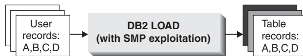
Figure 6. Record Order in the Source Data is Preserved When Intra-partition Parallelism is Exploited During a Load Operation
