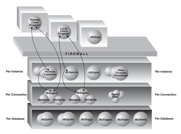
Figure 15. Process Model for DB2 Systems
