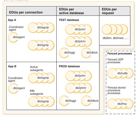
Figure 17. Process model, part 2
