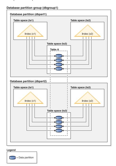
Figure 8. Index behaviour on a table that is both distributed and partitioned.
