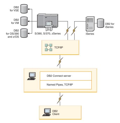
Figure 1. Connecting a client to a host or iSeries data server using DB2 Connect
