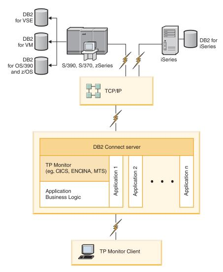
Figure 2. Transaction monitors working with DB2 Connect.
